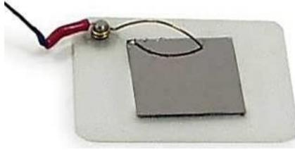
Fig. 9-2. Prepared substrate with a sample installed
