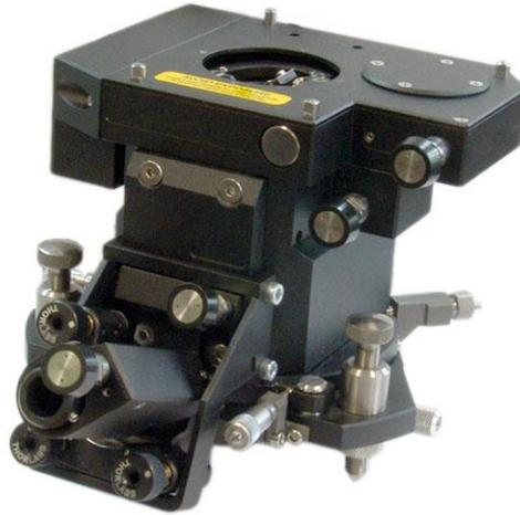
Fig. 2-15. Side illumination module installed on the measuring head
