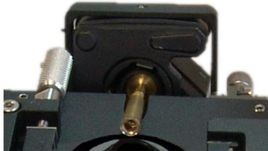
Fig. 8-16. Focusing module installed on the measuring head
