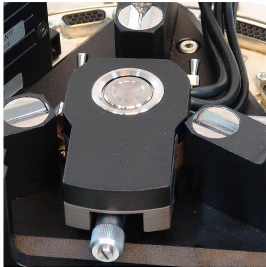
Fig. 7-3. Scanner installed in the positioning device
