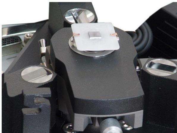
Fig. 8-5. Loading the sample into the scanner with sensors
