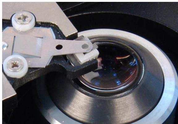
Fig. 8-21. Probe installed into the holder
