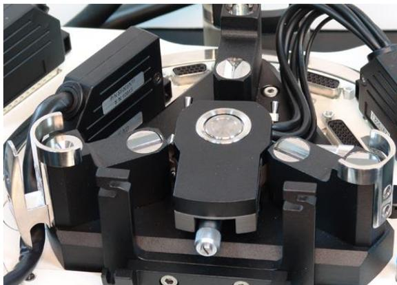
Fig. 2-3. Scanner with movement sensors mounted on the positioning device
