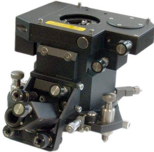
Fig. 8-15. Side illumination module installed on the measuring head
