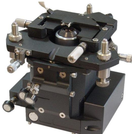
Fig. 9-5. STM tip holder installed
