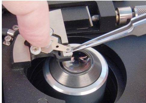
Fig. 8-20. Installing the probe
