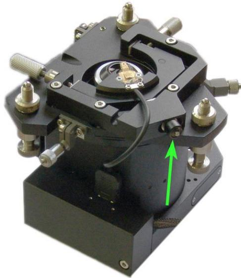
Fig. 8-17. AFM probe holder installed.
