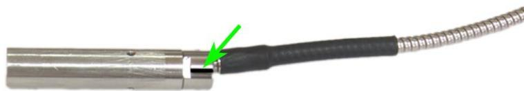
Fig. 2-20. **Output** socket.
