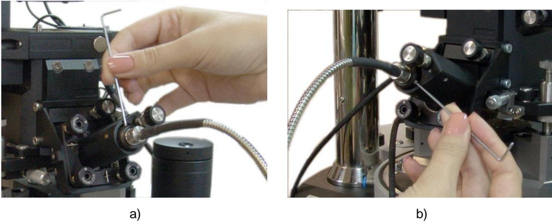
Fig. 8-26. Securing the **Output** socket
