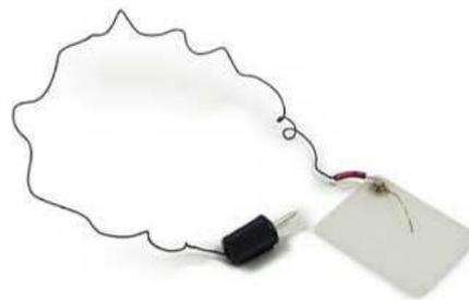
Fig. 8-9. Substrate with the spring contact
