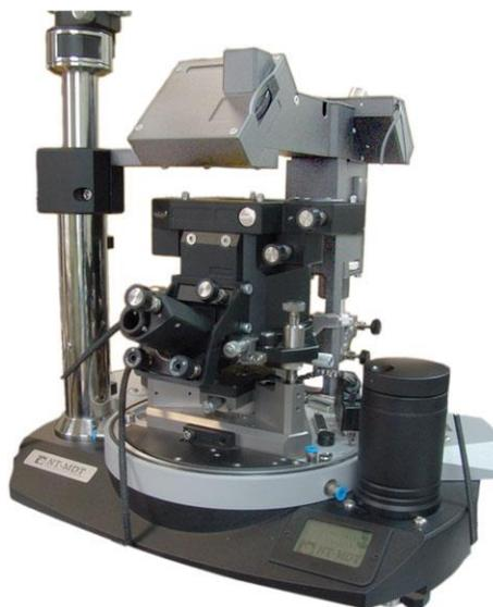
Fig. 8-23. Measuring head installed into the base unit
