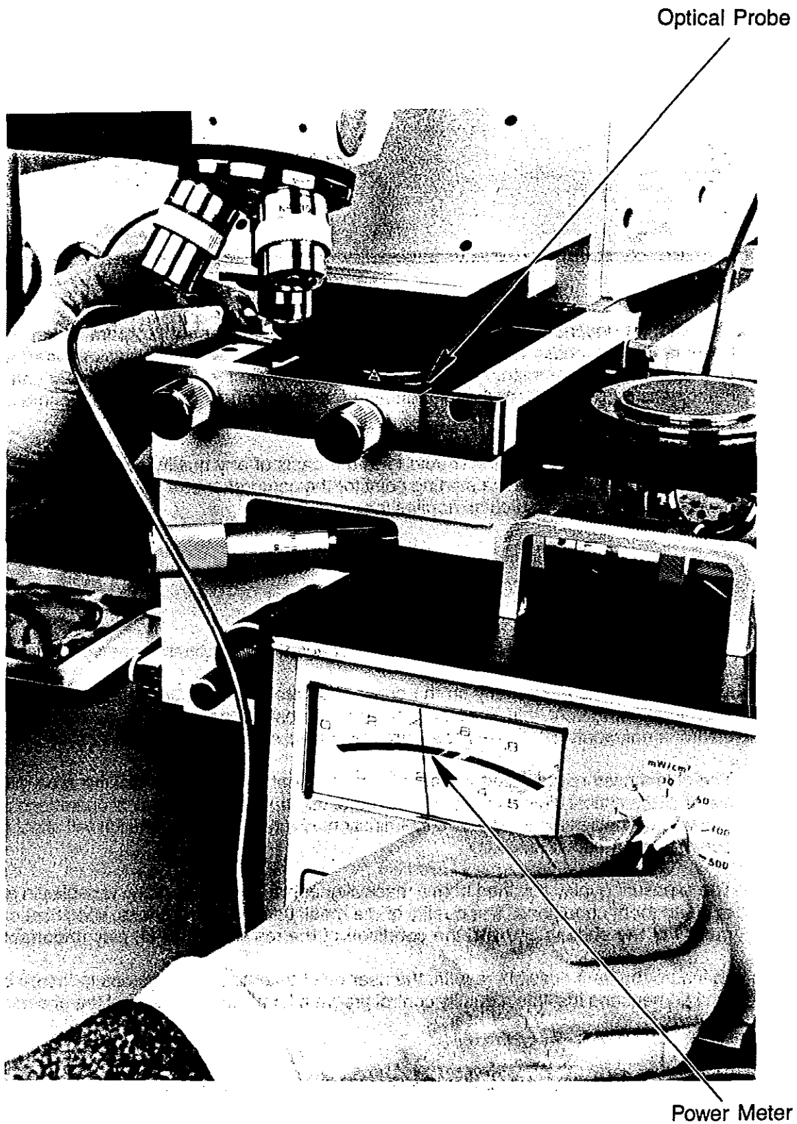
Figure 4-1 Measuring Light Intensity
